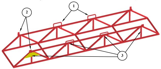
**Vertical rods** (3) shall be placed under every lifting handle / guiding device.
